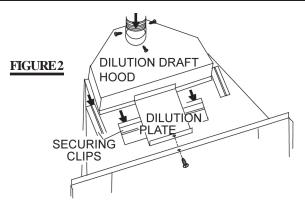
Line the chimney with a 3" or 4" diameter approved liner. With a 4" liner, an increaser must be connected between the dilution draft hood and the liner. Chimney installation must conform to both national and local code requirements. The liner must be continuous from the fireplace to the chimney cap.
